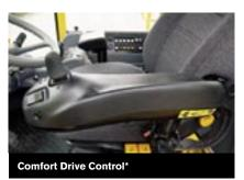
Significant reduction of repetitive and tiring steering wheel movements with CDC. Comfortable operation of steering and shifting with user-friendly controls in the left armrest.
